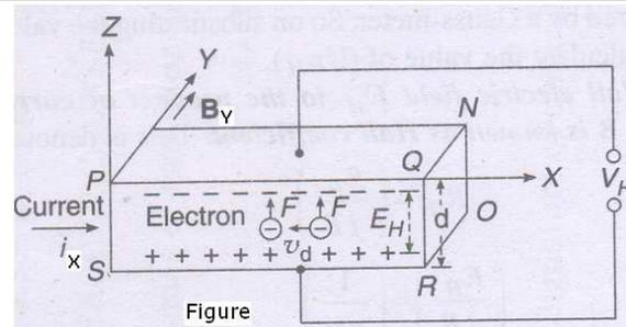
These  $F$  and  $E_H$  act in opposite directions. i.e. The forces due to magnetic field and electrostatic field on charge carrier act in opposite direction. Ultimately, the net force on the charge carrier becomes zero.
