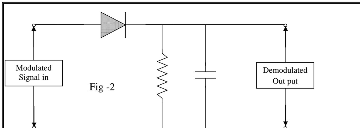
Amplitude demodulation circuit
